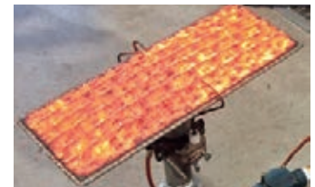
High-efficiency surface combustion gas burner
