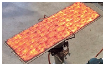
High-efficiency surface combustion gas burner
